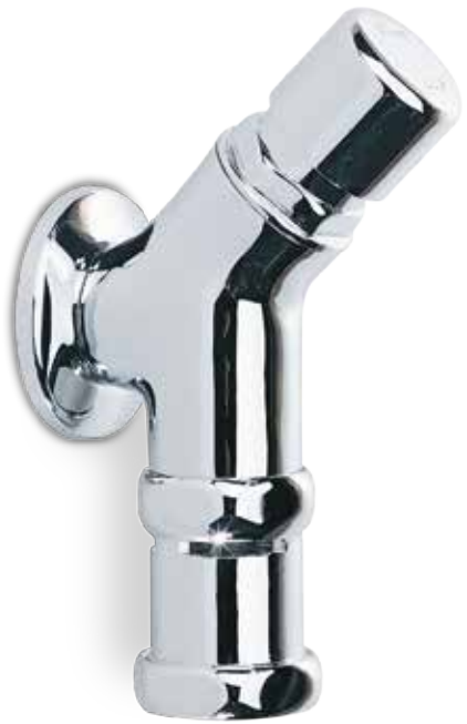
R 731 flussometro Ø 3/4" con dispositivo antisifonico incorporato erogazione per circa 6 secondi di 1,2 litri/secondo a 3 bar. External pushbutton operated flushometer with built-in anti-syphon device 28/30 Ø outlet 1,2 l/sec. supplied for about 6 sec. at 3 bar.
